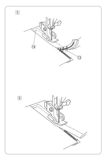
5 Raise and release the foot, and re-attach it with the left side pin.
