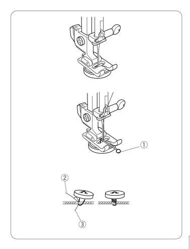
Unthread the needle. Adjust the stitch width to match it with the span of the holes in the button. Turn the handwheel to check if the needle enters into each hole in the button.
