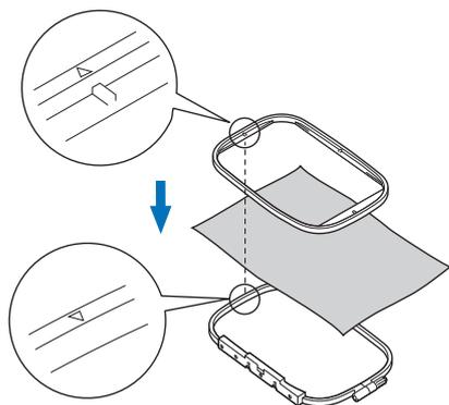
**4** Tighten the adjustment screw by hand just enough to secure the fabric.
