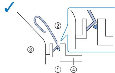
Notch (①) does not fit firmly under the bend in the lever (②).
