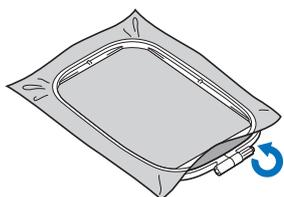
**5** Gently remove the fabric from the frame without loosening the adjustment screw.
