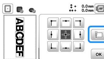
→ The needle is positioned in the lower-left corner of the pattern. The embroidery frame moves so that the needle is positioned correctly.
