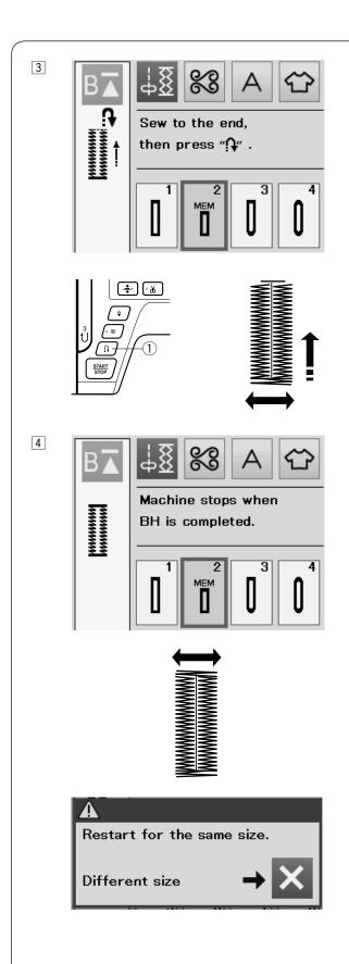
3 Start sewing again, and the machine sews the front bartack and right side of the buttonhole.
